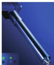
Cryostream, bio samples (Oxford Cryosystems Cobra)
