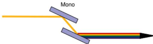
The mono is the device that turns white light (all energies) into monochromatic light (single energy).
