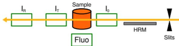
An ion chamber can also be used to measure the fluorescence signal. To increase efficiency (by increasing the signal-to-noise ratio), this detector is often used with a **slit assembly** and **fluorescence filters**.
