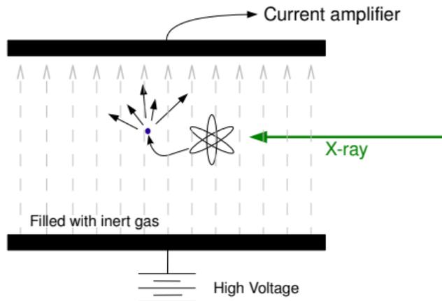
Flux on an ion chamber is easily computed
