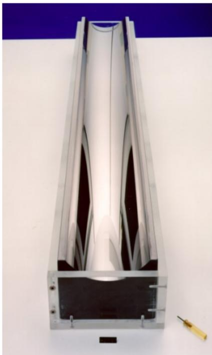
A toroidal mirror is bent lengthwise to focus vertically and is shaped in a circle to focus horizontally.
