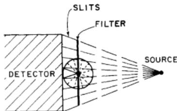
This sort of ion chamber is called a Stearn-Heald detector (diagram from EA Stern & SM Heald, *Rev. Sci. Instrum.* **50**, 1579 (1979)), also known as a Lytle detector.
