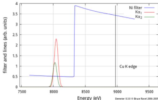
The filter material has its absorption edge between the energies of the incident beam and the dominant fluorescence lines of the sample.
