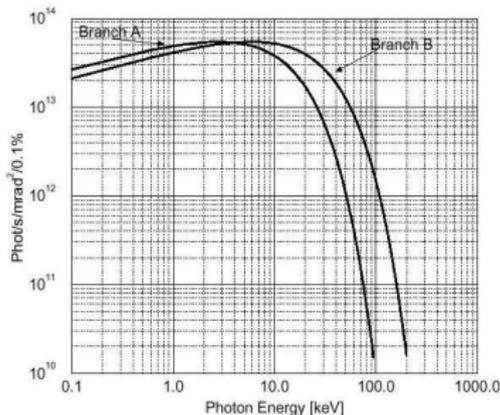
BM radiation has a characteristic energy  $\varepsilon_c$ , the *critical energy*, above which half of the total power is radiated:
