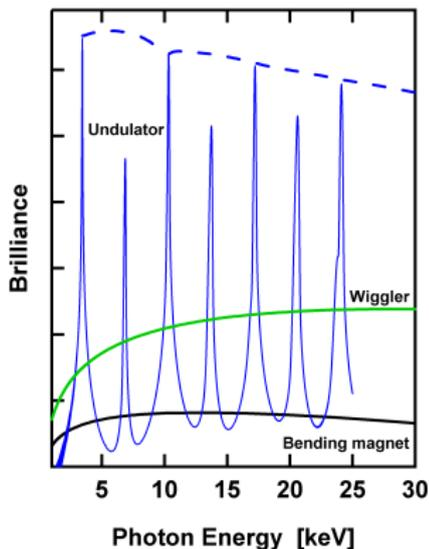
Undulators are much like wigglers, except the magnet period is shorter and the gap is often smaller. The light from each dipole is coherent, resulting in constructive interference at special wavelengths.
