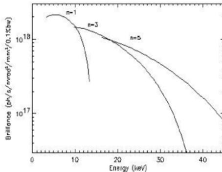
For a given gap, the undulator delivers extremely high intensity at discrete energies. To access other energies, the gap must be scanned.
