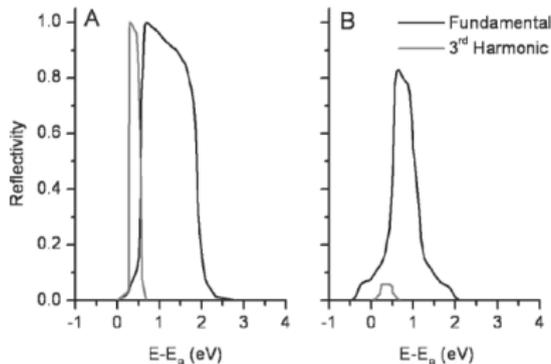
**Fig. 14-13.** Reflectivity of fundamental energy of 10 KeV and the third harmonic of 30 KeV from a Si(111) monochromator crystal as a change in relative energy from the Bragg energy ( $E_B$ ) (A) without detuning and (B) with a detuning angle of 3.5 arcsec. The intensity of the third harmonic in B has been multiplied by 100.
