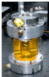
Gas flow reactor for redox chemistry
