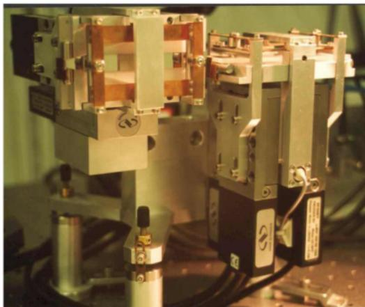
Depending on the details of the source, KB mirrors can focus from  $25\ \mu\text{m}$  to below  $100\ \text{nm}$ .
