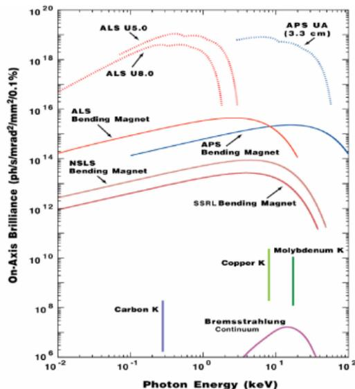
Photon properties produced by a synchrotron:
