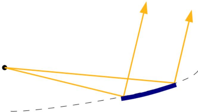
The VCM corrects the divergence of the beam, thus the instrumental resolution is defined by the mono crystal.
