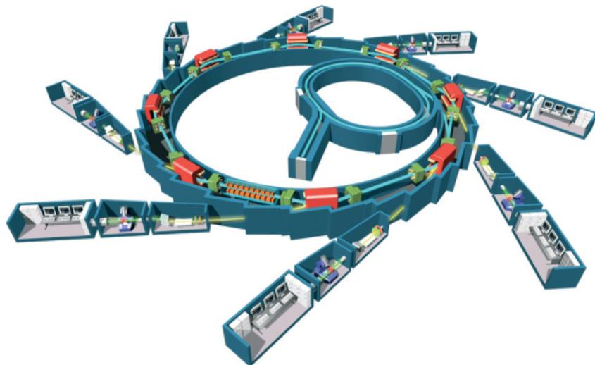
All synchrotron facilities have the same basic layout consisting of a storage ring with radiation emitted radially into beamlines. Beamlines consist of optics to condition the beam for experiments.
