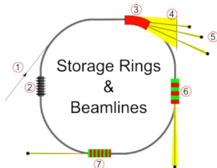
The storage ring is a large, evacuated, **polygonal** tube for containing relativistic electrons. Along with various kinds of magnets used to condition and shape the stored current, the ring has special magnets which generate useful X-rays as the electrons pass through.
