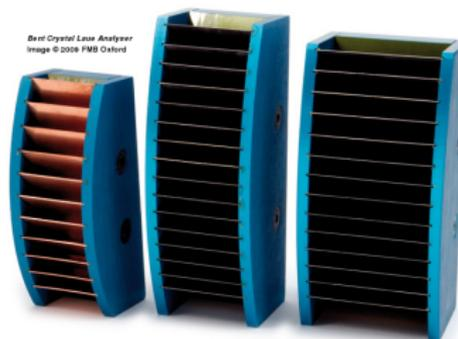
The bent Laue analyzer uses a thin silicon wafer bent over a frame. Rays of different energies Laue diffract in different directions from each other and from the transmitted rays. A filter assembly prevents all but the rays of the chosen energy from passing to the detector.
