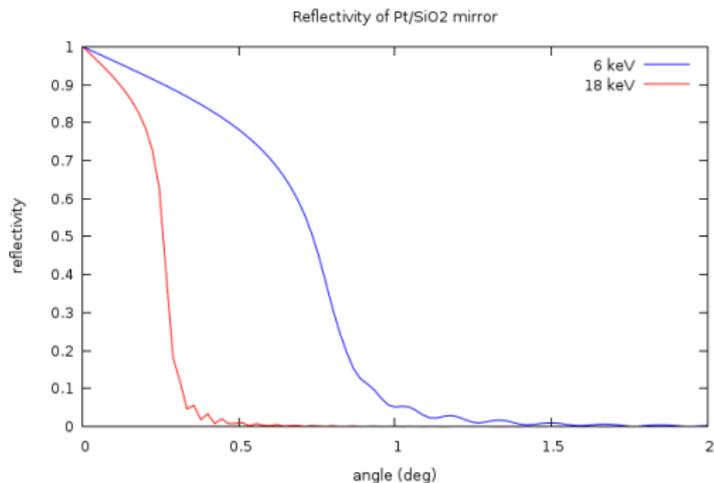
Setting a flat mirror to an appropriate angle (here, 0.5 deg) will pass most photons at 6 keV and absorb most photons at 18 keV.
