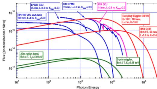
Figure 2. Flux vs. photon energy for various devices at NSLS-II.
