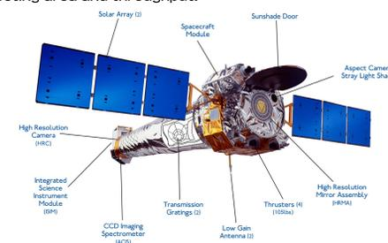
Chandra was launched and deployed by the Space Shuttle Columbia. It combines highly polished (a few Å rms roughness) nested mirrors with 4 scientific instruments (1) ACIS-S: array of 6 CCD cameras and (2) HETGS: high energy transmission grating spectrometer, our instrument of choice for XAS studies as it has the highest spectral resolution of any instrument currently flying. Also (3) HRC Camera: microchannel plates and (4) LETGS: low energy ...
