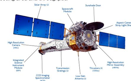
Chandra was launched and deployed by the Space Shuttle Columbia. It combines highly polished (a few Å rms roughness) nested mirrors with 4 scientific instruments (1) ACIS-S: array of 6 CCD cameras and (2) HETGS: high energy transmission grating spectrometer, our instrument of choice for XAS studies as it has the highest spectral resolution of any instrument currently flying. Also (3) HRC Camera: microchannel plates and (4) LETGS: low energy ...
