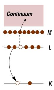
X-ray fluorescence and Auger emission occur at discrete energies that are characteristic of the absorbing atom, and can be used to identify the absorbing atom.
