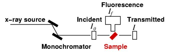
XAS measures the energy dependence of the x-ray absorption coefficient  $\mu(E)$  at and above the absorption edge of a selected element.  $\mu(E)$  can be measured two ways:
