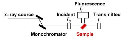
Scanning the x-ray energy across the Fe K-edge ( $\sim 7112\,\mathrm{eV}$ ), we measure the intensities of the incident beam and that transmitted through a sample (Fe<sub>2</sub>O<sub>3</sub>):
