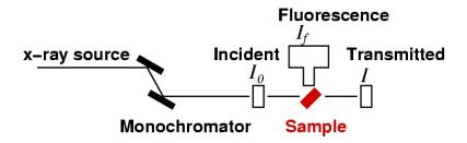
For concentrated samples, XAFS is best measured in transmission. To do this, we need enough transmission through the sample to get a decent signal for I. With,
