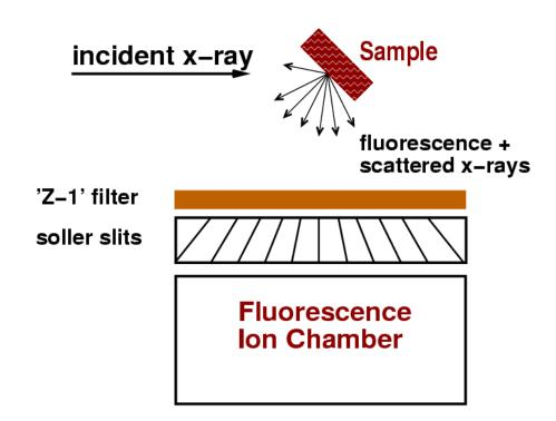
A set of Soller slits can be used to see the sample, but absorb most of the reradiate scatter from the filter.
