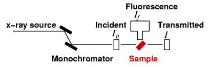
For thick samples or low concentrations (down to the ppm level), monitoring the x-ray fluorescence is the preferred measurement.
