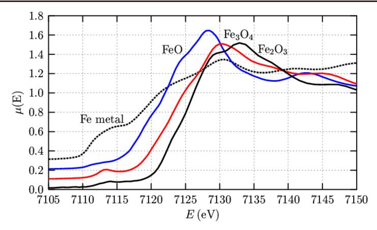
XANES for Fe oxides and metal. The shift of the edge position can be used to determine the valence state.
