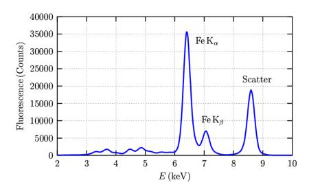
The x-rays emitted from the sample will include the fluorescence line of interest (here, both Fe  $K_{\alpha}$  and Fe  $K_{\beta}$ ) as well as *scattered* x-rays, and other fluorescence lines (here, Ca, Ti, and V).
