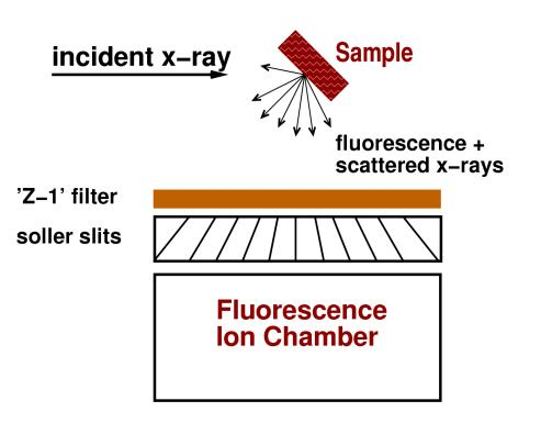
A set of **Soller slits** can be used to see the sample, but absorb most of the reradiate scatter from the filter.
