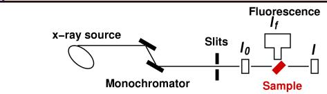
For thick samples or low concentrations (down to the ppm level), monitoring the x-ray fluorescence is the preferred measurement.
