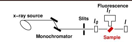
Scanning the x-ray energy across the Fe *K*-edge ( $\sim 7112 \text{ eV}$ ), we measure the intensities of the incident beam and that transmitted through a sample (Fe<sub>2</sub>O<sub>3</sub>):
