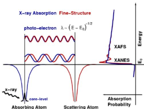
The scattering of the photo-electron wave function interferes with itself.
