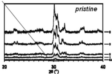
GIXRD measurements of the pristine zirconolite surface show that crystalline structure persists to the surface.
