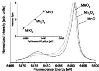
Energy analyzing the fluorescence lines yields information about the electronic structures of different chemical states.
