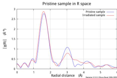
The structural changes observed at the Zr K-edge are much more subtle. There is a slight red-shift of the edge energy, a slight shortening of the Zr–O bond, and an increase in higher shell disorder.
