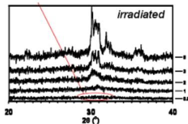
After heavy ion bombardment, the bulk crystallinity vanishes near the surface.
